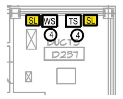
A4. These are intended to be control modules as required by the riser diagram on drawing FA-601.
